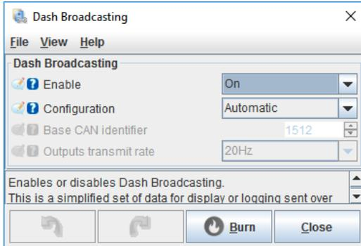
To display ethanol content, the “CAN Realtime Data Broadcasting” must be enabled. Go to “CAN bus/Testmodes menu and select “CAN Realtime Data Broadcasting”. Set “Enable realtime...” to ON and set the “Base message identifier” to default value (1520). Then set a “Broadcasting rate” to 10hz.
